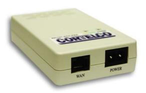
The ATA-100 is an analog telephone adapter that connects an analog telephone device to an IP network, enabling SIP-supported VoIP communication in applications where connecting to an existing FXS port is not possible or practical. In addition, the ATA-100 has an RJ-11 port for switching to the PSTN analog phone network via touch tone commands.
